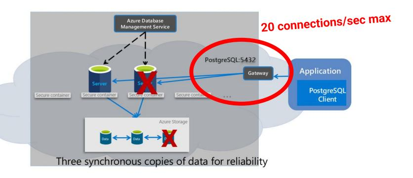
Single point of failure DB replicas
